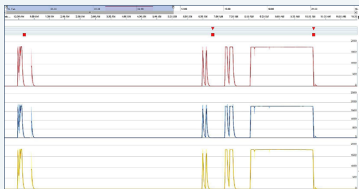
Figure B. DriveScan's patented DC cell capacitor monitoring showed no significant variation between phases on the DC bus. Keep in mind that after a fault, the drive's input contactor opens, removing power from all the cells.
