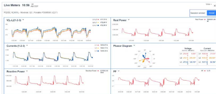
Figure 1: Data pulled from live meters. Every two minutes, the aluminum extrusion pressing cycle occurred, as seen in current peaks, voltage drops, and increases in power factor and kVAR. Such data proved instrumental in understanding the application and load.
