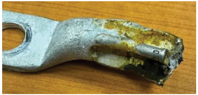
Figure 3: A poorly implemented, nonuniform crimp on the cable termination caused discoloration and was the culprit of electrical discharges that would've led to cable failure
